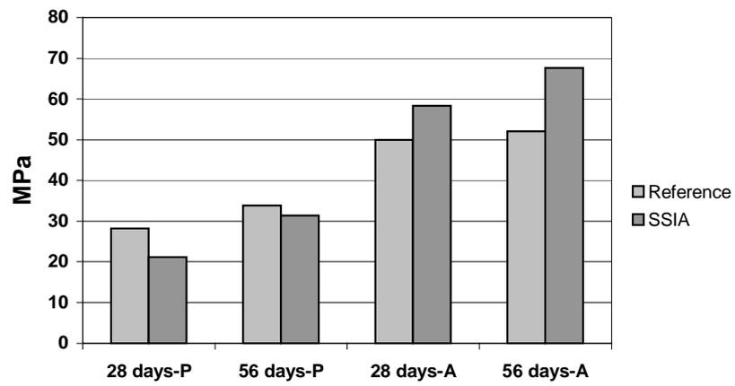
Fig. 3. Strengths for reference concretes and concretes with SSIA for passive and aggressive environmental class. P: Passive environmental class, A: Aggressive environmental class, SSIA: Sewage sludge combustion ash
