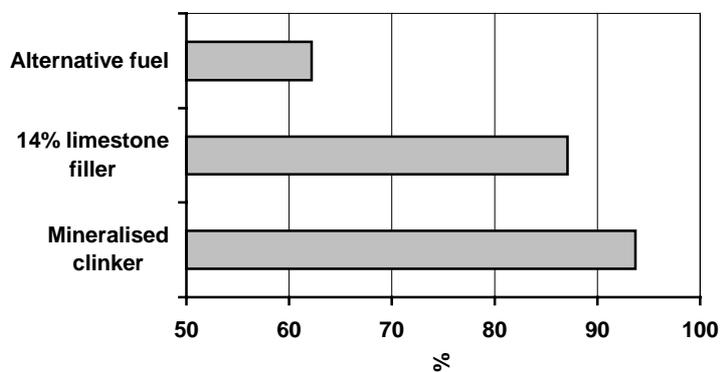
Fig. 2. CO<sub>2</sub> reductions (excl. calcination) expected after present research and development is fully implemented in Aalborg Portland's cement production. 100% = CO<sub>2</sub> emission from Aalborg Portland's largest cements kiln during conventional cement production.
