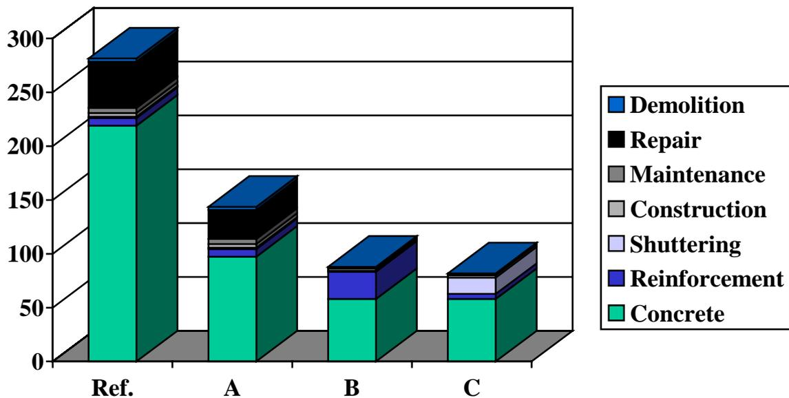
Figure 1 Sources of CO<sub>2</sub> emission for four types of columns
