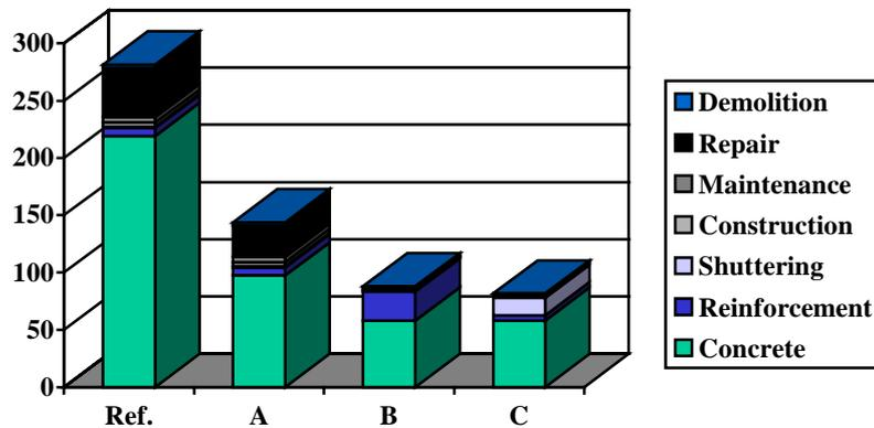
Figure 2 Sources of CO<sub>2</sub>-emission for four types of columns
