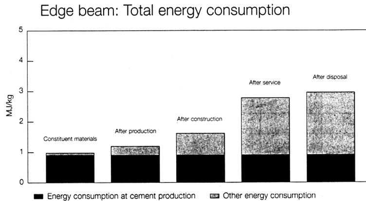
**Figure 1. Edge beam: Total energy consumption through all the life cycle phases (2)**
